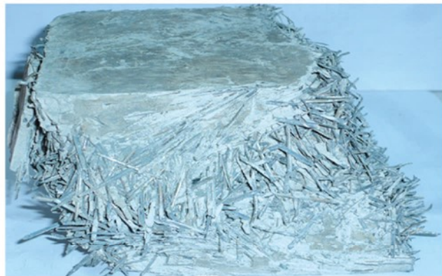
试块受压后的形貌 Shape of test block after compression
