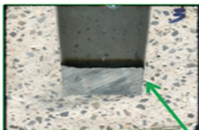
BA-80浇注料的抗铝效果 The result of osmosis-resistant castable BA-80
