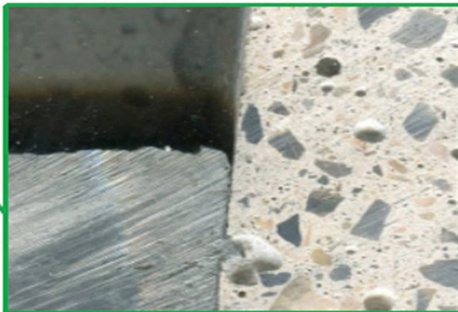
BA-80浇注料的抗铝效果 The result of osmosis-resistant castable BA-80
